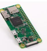
The low-profile (2.6" x 1.2" x 0.2") Pi Zero technically has a full-size GPIO header, but the pins have to be soldered on by the user if they are needed.
